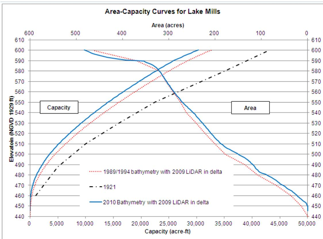
Figure 1. Example area-capacity curve for Lake Mills Reservoir on the Elwha River, Washington State generated with a GIS-based approach.
