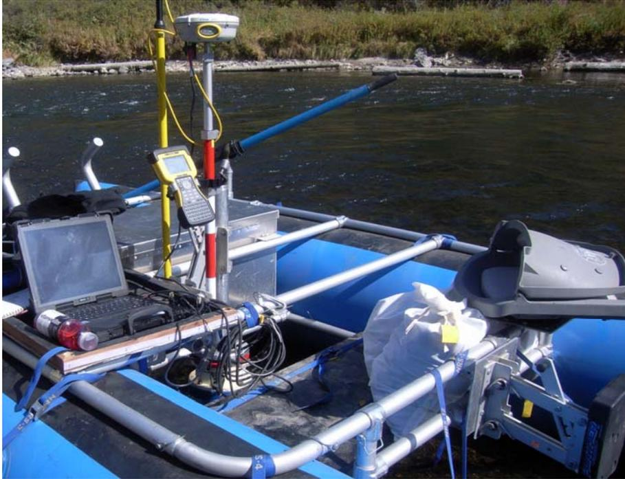
Figure 3. Example bathymetric equipment setup with RTK GPS, ADCP, and laptop on river cataract for shallow reservoir areas or riverine segments. Photography courtesy of Sedimentation & River Hydraulics Group, Reclamation, Denver, Colorado.
