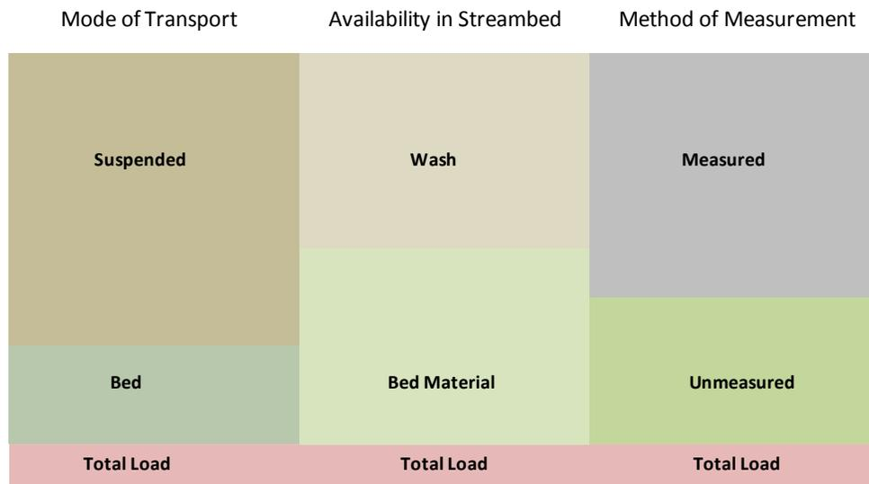
Figure 4. Different Classifications of Total Sediment Load (after USACE, 1995a)
