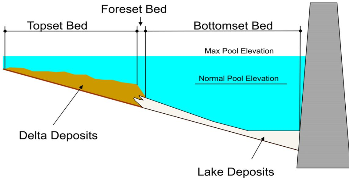
Figure 5. Conceptual View of Reservoir Deposition Zones
